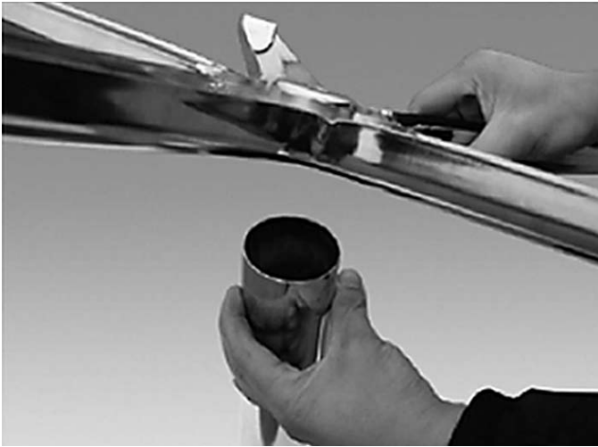
Step 3: Place table base over end of the column as shown in picture.
