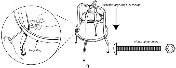
STEP 4: Set the swivel on the top of the finished frame. Align the bottom set of holes (the side closest to the frame) with the holes in the frame. Insert the medium size bolts from the top (through the
