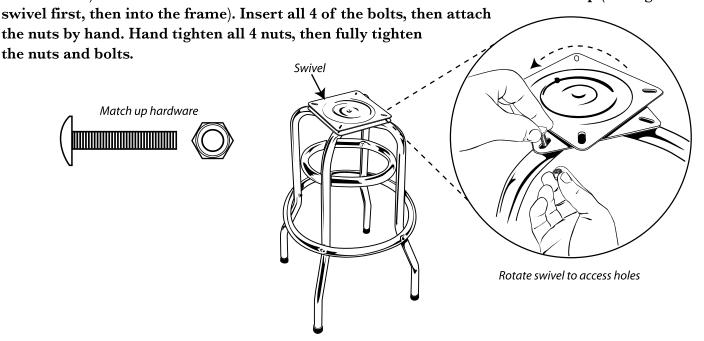
STEP 5: Place the top of frame swivel assembly onto the seat bottom, and align the holes. Insert all 4 bolts (smaller size) part way, then fully tighten. Set your Bar Stool right side up and enjoy!
