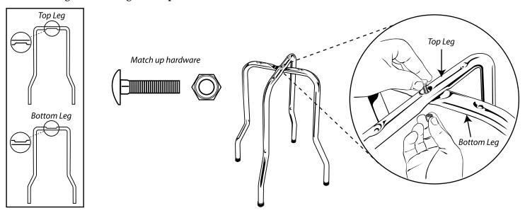
STEP 2: Slide the small ring up under the legs and align the screw holes. Insert the medium size bolts from the inside (through the ring first, then into the legs). Insert all 4 bolts
