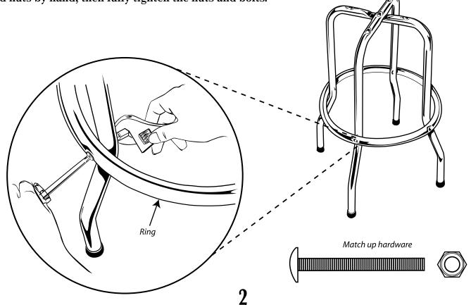
STEP 3: Set the swivel on the top of the finished frame. Align the bottom set of holes (the side closest to the frame) with the holes in the frame. Insert the medium size bolts from the top (through the swivel first, then into the frame). Insert all 4 of the bolts, then attach the nuts by hand.
