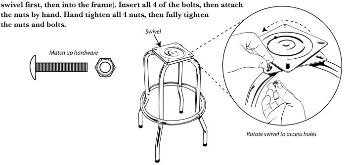
STEP 4: Place the top of frame swivel assembly onto the seat bottom, and align the holes. Insert all 4 bolts (smaller size) part way, then fully tighten. Set your Bar Stool right side up and enjoy!
