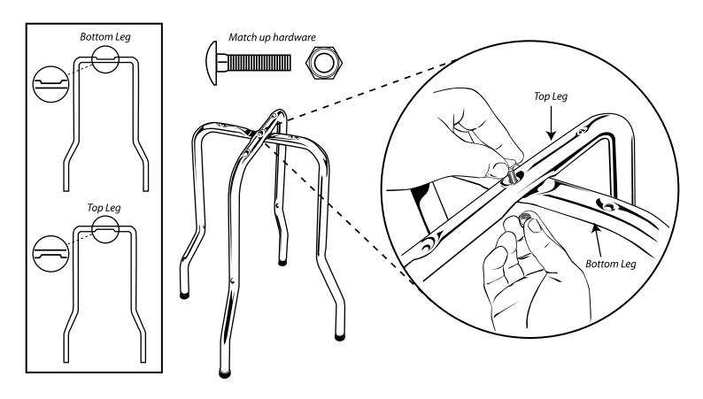
STEP 2: Slide the ring over the top of the legs and align the screw holes. Insert the long size bolts from the outside (through the ring first, then through the frame). Insert all 4 bolts and nuts by hand, then fully tighten the nuts and bolts.
