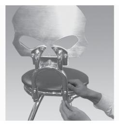
**Step 8:** Securely fasten the billet backrest to the seat base using small bolts and tighten securely.
