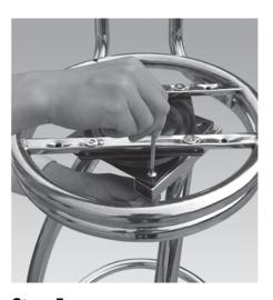
**Step 5:** Flip over and attach swivel plate to bar stool legs. Use large bolts with lock nuts. Tighten securely.
