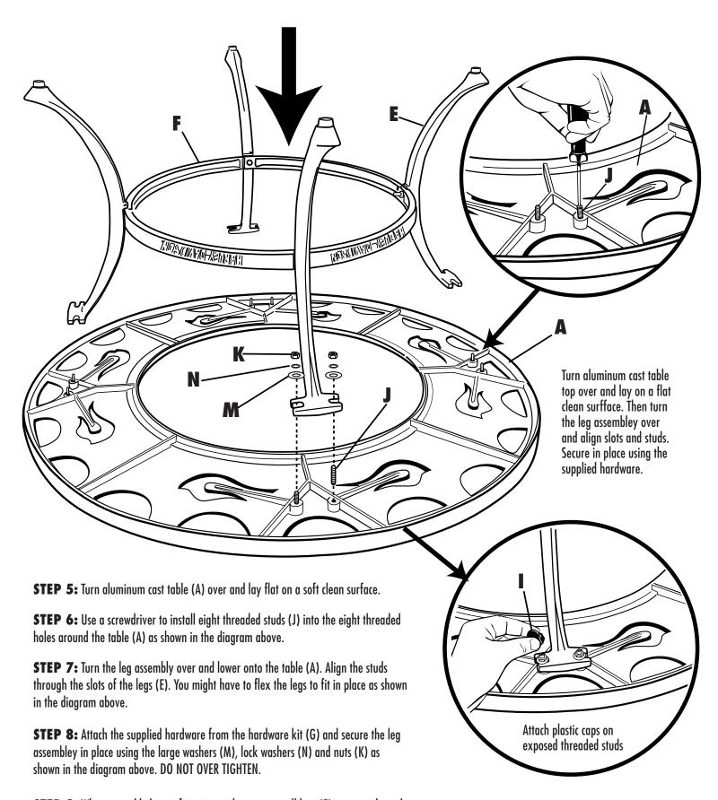
**STEP 9:** When assembled, turn fire pit upright to ensure all legs (E) are straight and the table surface is level then fully tighten all huts (K).
