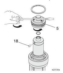
3. **Series B and later T2 pumps:** Unscrew air valve (5). If necessary to assist turning, wedge a screwdriver blade between the screw heads and the hex cap of the air valve (5).
