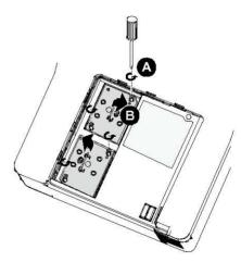
**3.** Pull firmly on the module handle in the direction shown to remove the lamp.
