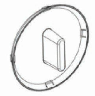
LENS HOLE CAP (INSTALLED)
