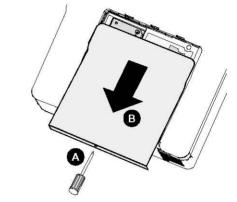
**3.** Unscrew the retaining screws (x 4) on the four-segment color wheel.
