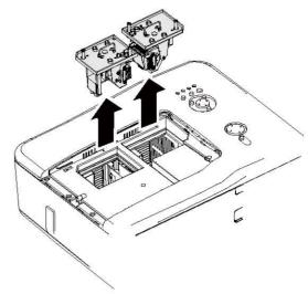
4. Reverse steps 1 to 3 to install the new lamp module(s) and replace the lamp cover.
