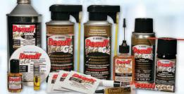
**DeoxIT® Gold G-Series** is a unique formulation which conditions, seals, and protects gold plated metal connectors and contacts. **DeoxIT® Gold** is ideal for gold and all nonferrous metal surfaces. It deoxidizes minor amounts of surface contamination, penetrates plated surfaces, and molecularly bonds to the base metal, sealing and protection all surfaces.
