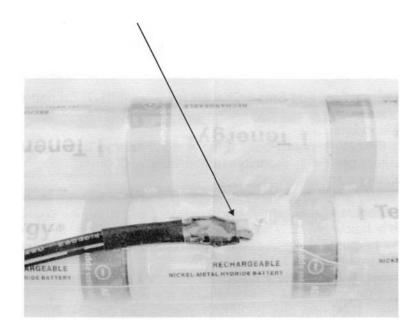
Step 1: Put the temperature sensor onto the middle surface of battery pack.
