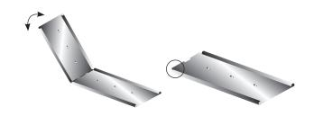
When snapping plates to length ensure edges do not curl up as this can damage tube. Flatten with a hammer or grips.
