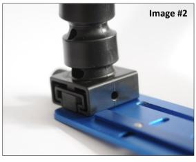
d. After tightening the screw, in order to ensure that the arm is completely locked, try to push it out of the tray by gliding the Flex Arm's C1 connector in the opposite direction to the one used to glide it in. If the Flex Arm comes out, repeat steps 1-3 again and make sure that the C1 and T1 connectors are perfectly aligned prior to tightening the screw.
